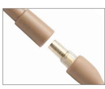
*Sweat-Resistant Connector:* The mic detaches from the cable using a new connector with a tight seal against moisture (e.g., sweat).
