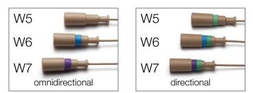
*Three Sensitivity Options:* The H6 Headset has three sensitivity options. Choose W5 (no band) for general speaking, W6 (blue band) for loud speaking and vocals, and W7 (purple band) for powerful vocals such as opera. Directional microphones are marked with an additional green band.
