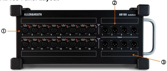
U Input sockets 16 balanced XLR mic/line inputs with +48V Phantom Power indicator. The preamps are built into the AB168 and their Gain. Pad and 48V phantom power are remote controlled from the mixer via the dSNAKE link. The outputs of the analogue preamps are converted to digital format and transported via dSNAKE to be processed and mixed at the GLD or Qu mixer.
